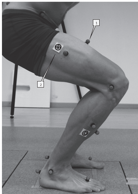
Squat knee-angle measurement with Vicon Motion Systems markers (1) and CSEM 6D tags (2)
