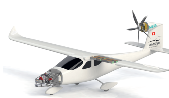
Batteries, combustion engine and electric motor placed inside the airplane.
