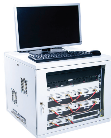
Hardware of the indoor localization system
