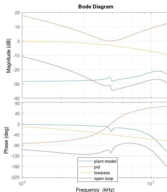
The plant model with the pid and a second order lowpass gives the open loop response.
