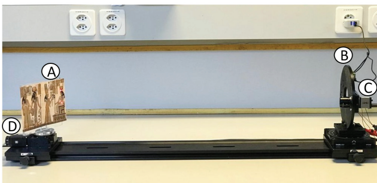
A) Historical image, B) Prototype of the system, C) Small camera, and D) Stepper motor to rotate the image
