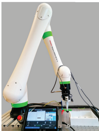
Figure 1 : Prototype set-up with a Fanuc CRX-10iaL Cobot.
