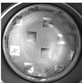
Coffee capsule: Coffee particles in the sealing seam
