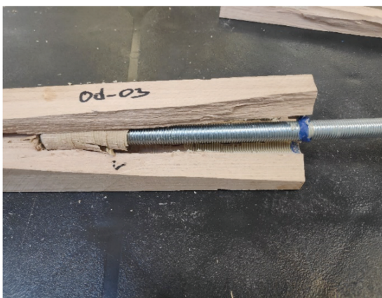
Figure 1: Timber splitting failure
