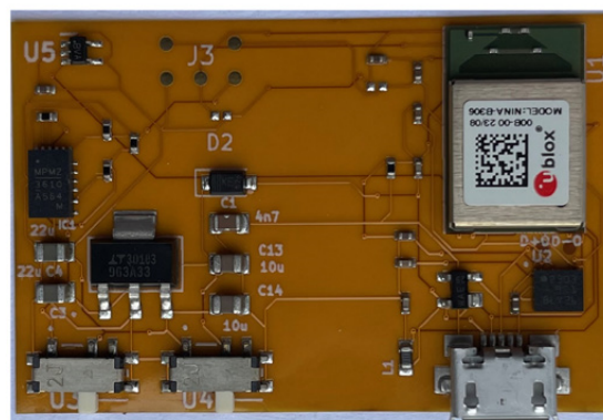
Figure 2: Top view of the circuit realized to make the handpiece connected. Dimensions: 44 mm x 29 mm
