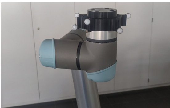
Figure 1: Markers for Robot Flange
