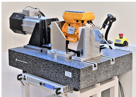
Motor test bench, equipped with an ennos slp2 0.5Hp motor.
