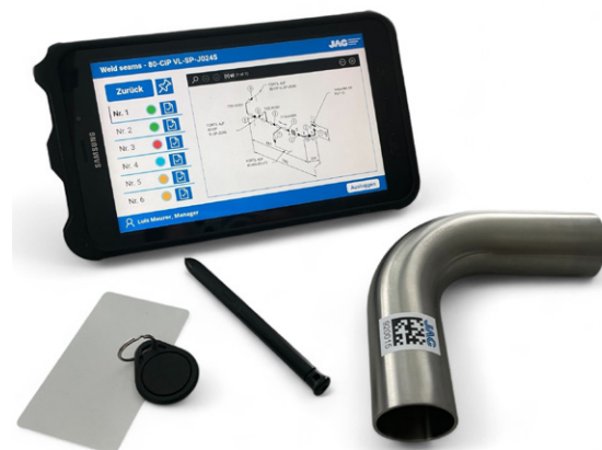
Figure 2: Prototype application with NFC tags and Matrix code on a pipe, that will be welded into a pharmaceutical plant.
