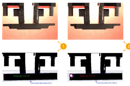
Figure 2: Images from the external camera. Top: Raw image. Below: Inspection results, (1) good part, (2) defective part.
