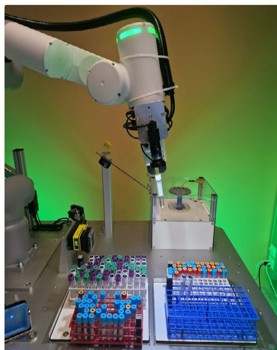
Figure 2: The cobotic cell demonstrating lab automation tasks
