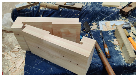
The traditional longitudinal wood joint Kanawa-Tsugi crafted in manual joinery (Model)
