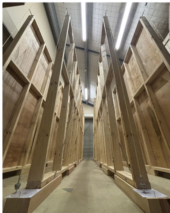
Test frames installed in the test cell for long-term distortion assessment
