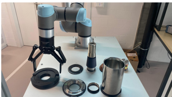
UR5e robot assembling a X-ray tube
