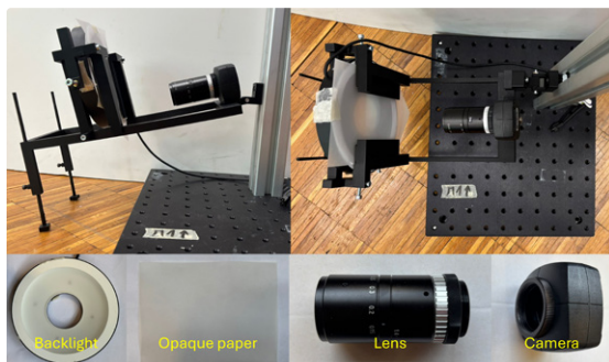
Fig. 1: Test setup for real components with integrated camera and backlight. Top left: side view. Top right: top view.
