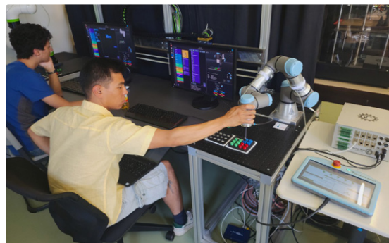
Electronics apprentice programming a pick-and-place task with a cobot.
