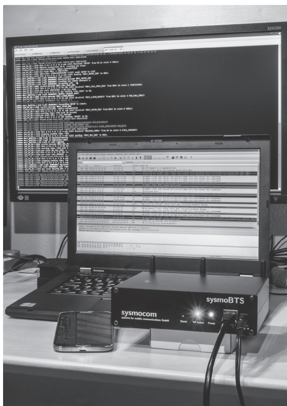
My set-up to monitor GPRS IP traffic on a sysmoBTS with Wireshark.
