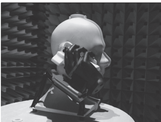
S4 inside OTA-Chamber, reference Beside Head Hand Right (BHHR)
