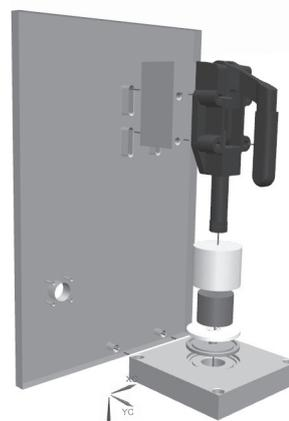
Assembly of principales parts of the source
